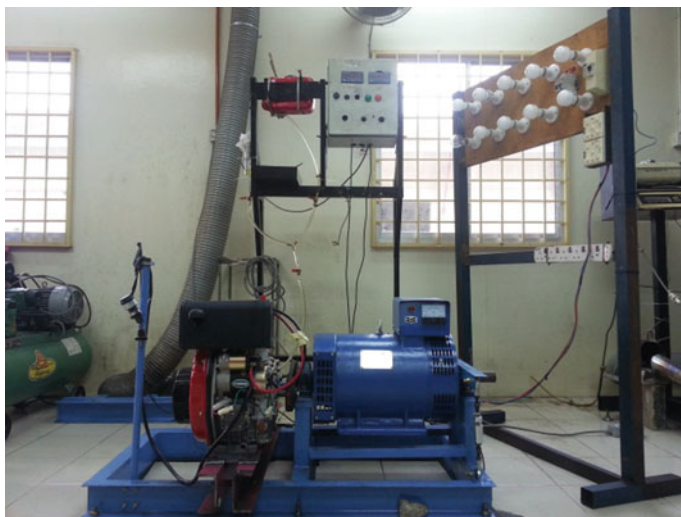
Fig. 1 Yanmar 178F CI engine performance experimental setup
