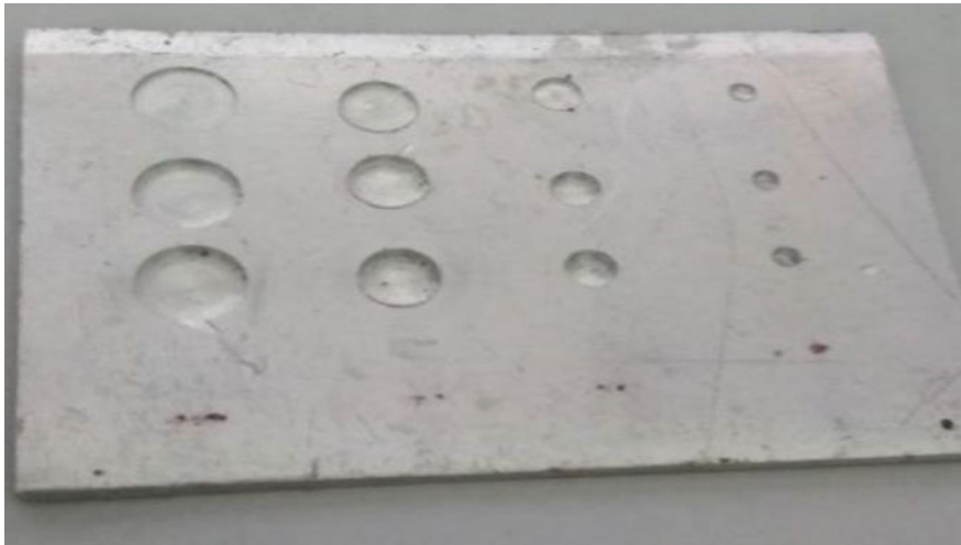
Fig. 3 Actual specimen used in the thermography test
